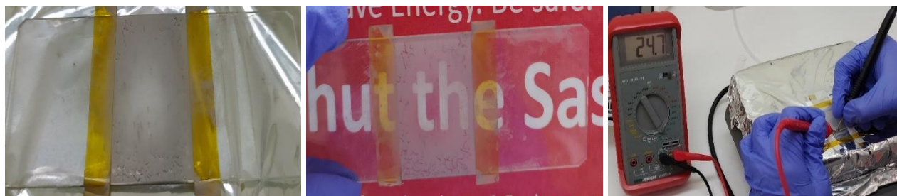
Figure 6.1 – Spray coating process on a glass substrate and measuring of its electrical resistance with a multimeter.
