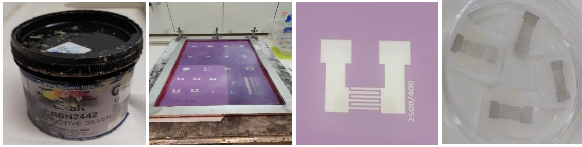
Figure 3.11 – Materials and method used to fabricate the IDEs on the membrane surface and the resulting product.
