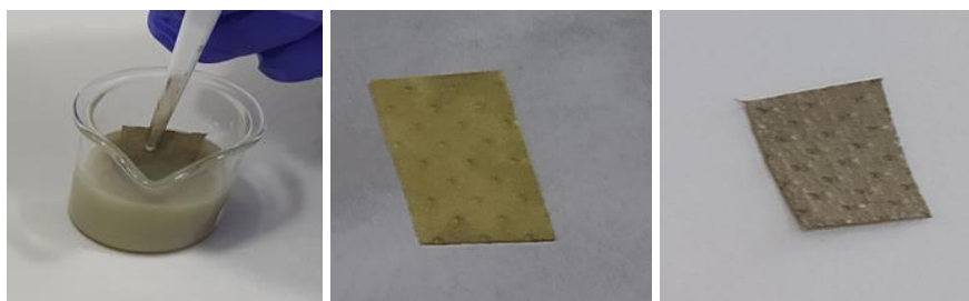
Figure 3.18 – The dip coating process on the paper Tork and its appearance with the AgNWs before and after annealing.
