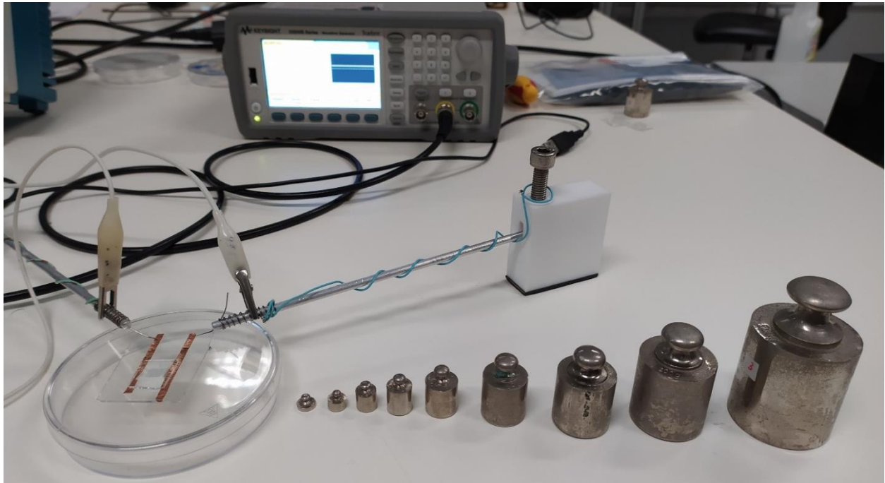
Figure 6.9 – Setup (sensor, probes and the KEYSIGHT 33500B series waveform generator) with the weights used during the sensitivity tests to apply specific pressures on the sensor.
