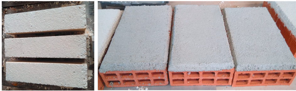
Fig. 1. Examples of prismatic and render on brick mortar samples produced.
