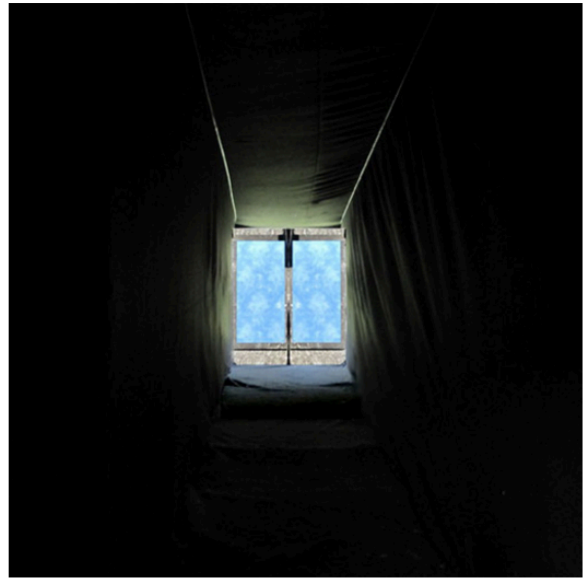
Figure 2: A bird's view from inside ABC's Powdermill Test Tunnel, with clear glass on the left, glass with vertical stripes on the right. Note the net, which prevents birds from actually contacting the glass.
