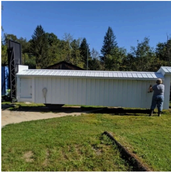
Figure 1: The Powdermill tunnel in operation. Birds are placed into the tunnel through a sleeve, at the right end, where video camera and computer are also located. The release door can be seen at the left end of the facing side of the tunnel. Glass is mounted outside the right end of the tunnel.
