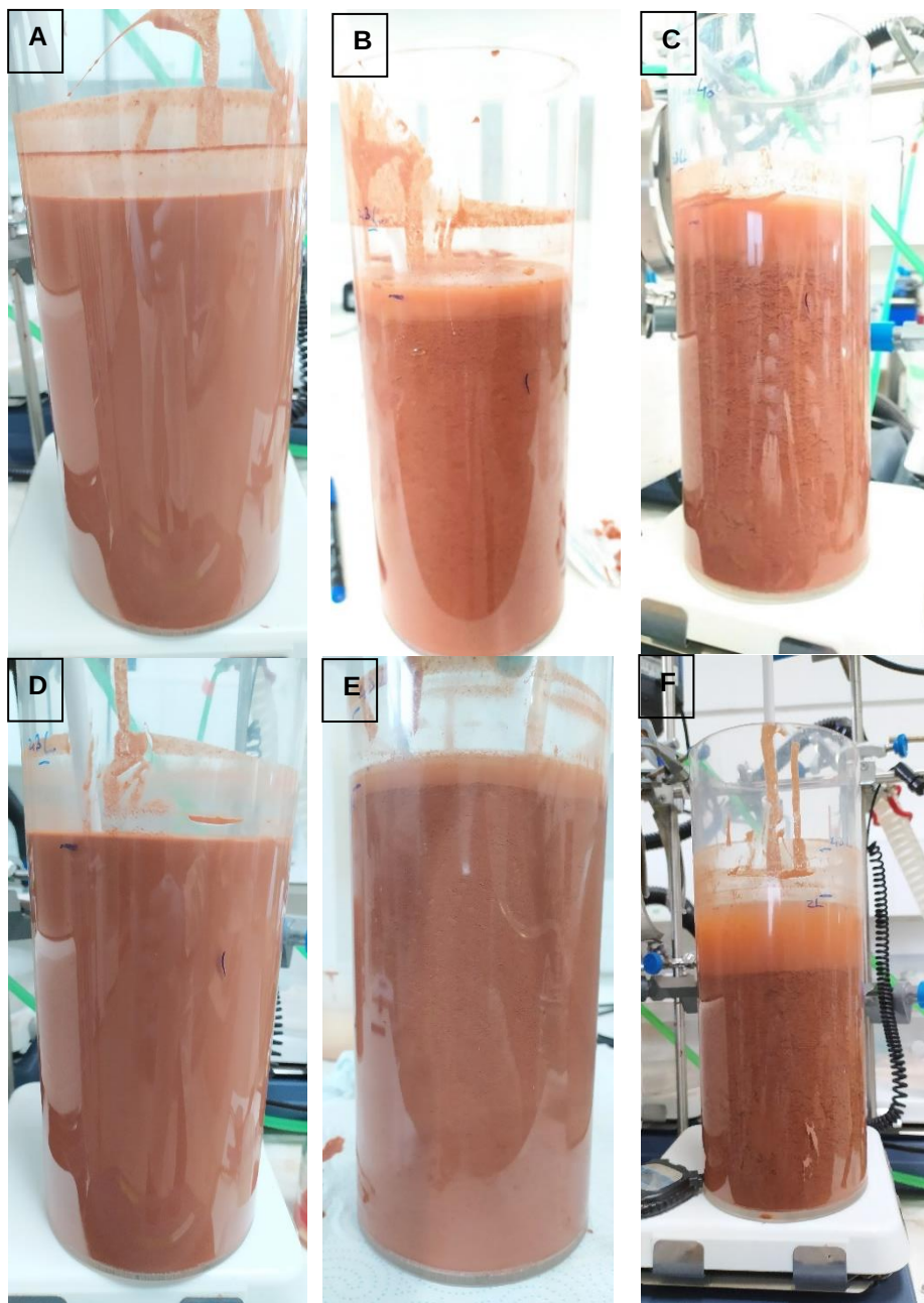
Figure 3.25 – Side by side comparison of solutions treated with \text{Al}_2(\text{SO}_4)_3 at: (A) – 200 mg/L; (B) - 1000 mg/L; (C) – 1500 mg/L and PFS at (D) – 200 mg/L; (E) – 1000 mg/L; (F) – 1500 mg/L
