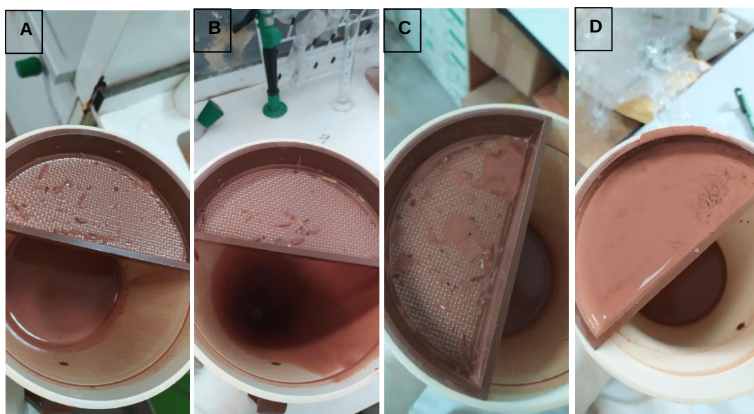
Figure 3.6 - Deposits retained on the net of the Marsh funnel for 24 minutes mixing time and different concentrations of \text{Al}_2(\text{SO}_4)_3 : (A) – 5 mg/L, (B) – 50 mg/L, C – 200 mg/L, D – 600 mg/L
