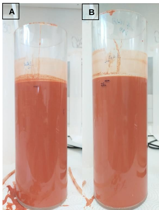
Figure 3.51 – Side view of the solutions treated with (A) – NaCl + Microbond and (B) – NaCl + 6610
