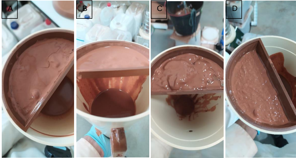
Figure 3.18 - Deposits retained on the net of the Marsh funnel for: (A) - single level agitator, 200 rpm; (B) - single level agitator, 300 rpm; (C) - two level agitator, 200 rpm; (D) – two level agitator, 300 rpm at 600 mg/L
