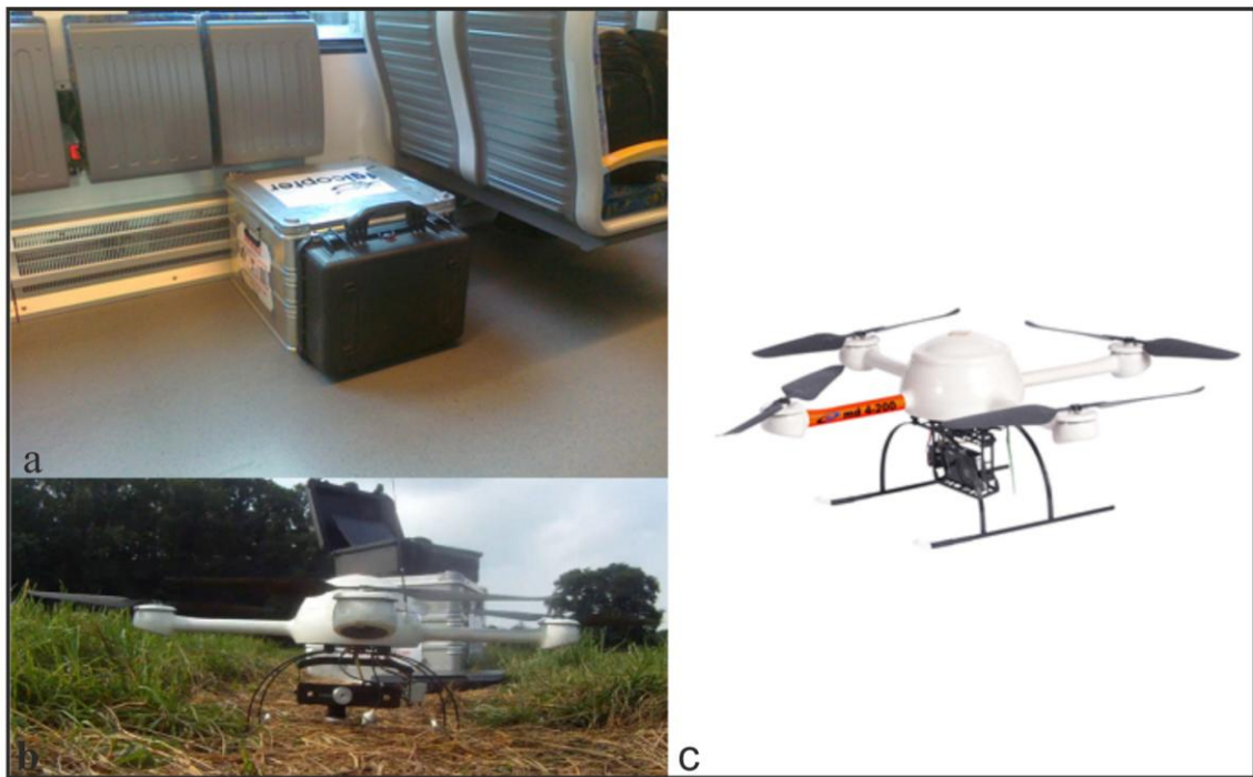
Figure 12. a) quadrocopter microdrone md 4-200 and ground station in transportation boxes, b) quadrocopter microdrone md 4-200 and ground station with modified digital camera (Canon PowerShot SD 780 IS), c)quadrocopter microdrone md 4-200 (Microdrone 2014).
