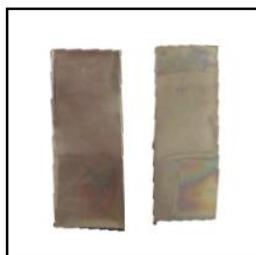
Figure 3.37: Chitosan films of 4 layers made with solutions B (left) and C (right).
