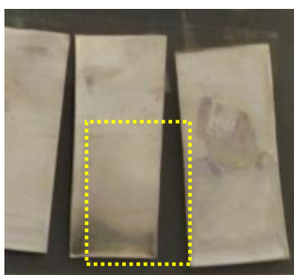
Figure 3.43: Films deposited with a solution of PCL 1.95 % wt/v in DCM with the film covered area detailed in yellow.
