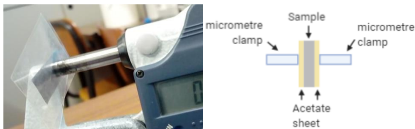
Figure 2.14: Setup used to measure film thickness showing the placement of micrometre clamps, acetate sheet and sample.
