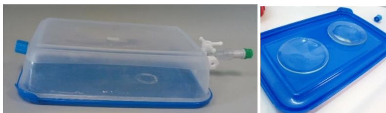
Figure 2.12: Recipient used for silanization in Ar atmosphere with detail on TEOS and ammonium recipients on the right.
