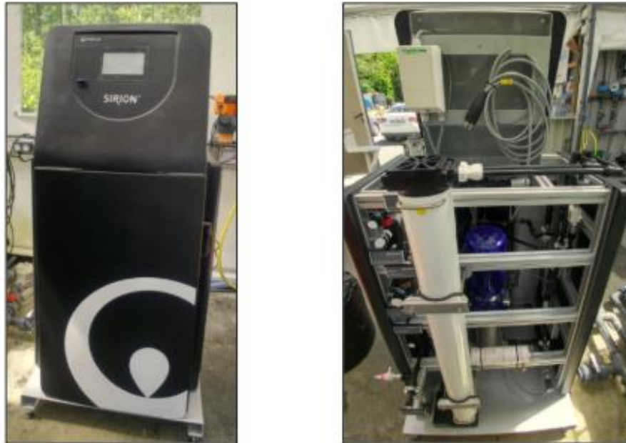
Figure 20: RO ReUse pilot
